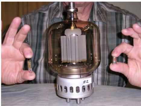
The tube on the left is a sub-miniature "pencil" tube used in portable receivers in the 1960s. These tubes, made by Raytheon, were competing with the early transistor sets. We know who won and the pencil tubes were phased out. They used very little filament and plate operating power.
