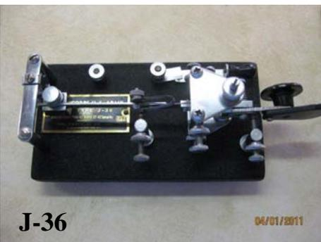
This bug is the Vibroplex J-36. The label says Signal Corps-U.S. Army. The serial number is 1673. It has a contract date of June 27, 1942. I am not sure what that means since these were manufactured from 1941-1945. It might mean that
